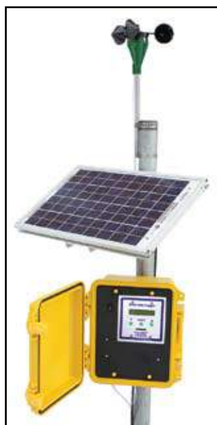
#2: A professional-grade logging anemometer. Photo courtesy of APRS World www.aprsworld.com
